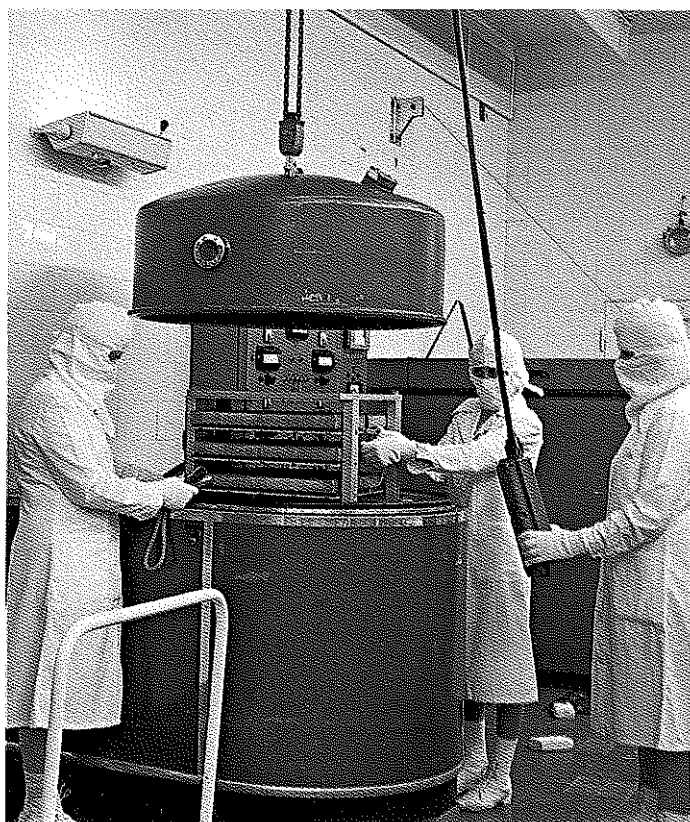
Human (Gödöllő) — Freeze-drying (liophylization) of human blood plasma albumin
