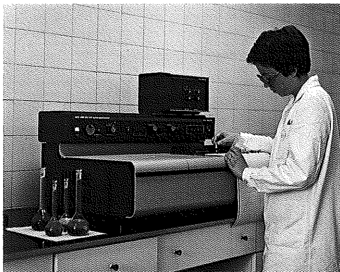
State Pharmaceutical Institute (Budapest) — Examination of drugs by spectrophotometry
